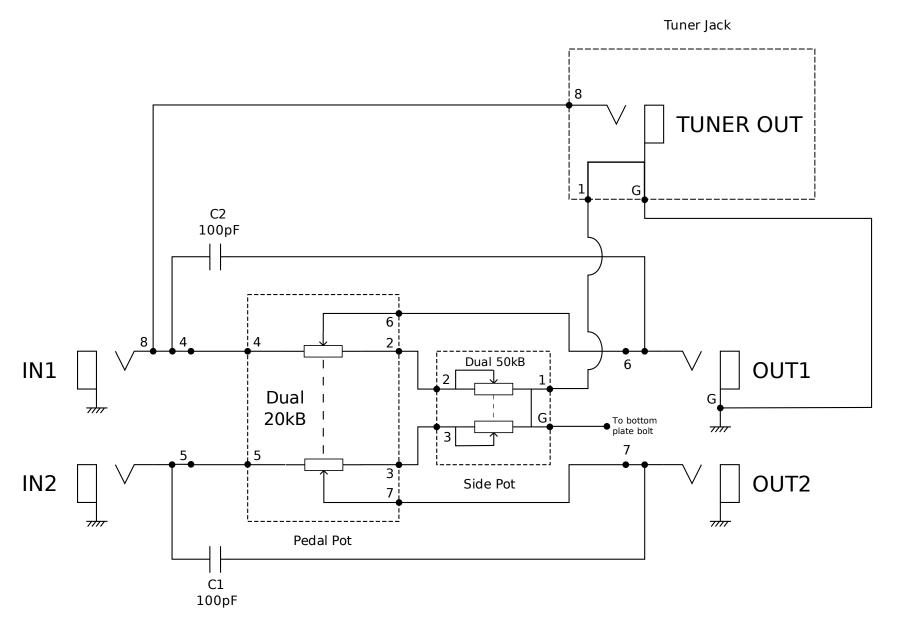
Dotted line show the different boards inside the unit. Main board not shown. Numbers/letters and components according to the PCB.
