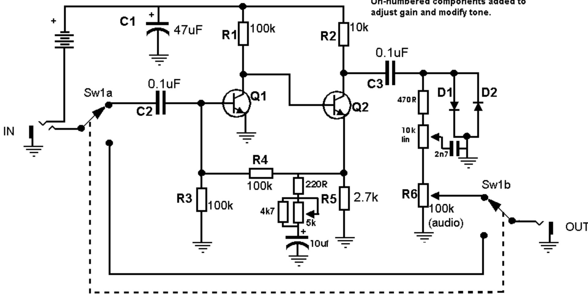
This is the Muff Fuzz with true bypass switching. The transistors are 2N5088 or 2N5089 and the diodes are 1N914/1N4148 or 1N34A.
