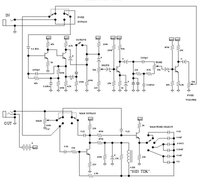
The Foxx Fuzz Wah includes a fuzz, an octave effect, a wah pedal, and in later versions a volume pedal all in the same box. The box, by the way, is covered in blue or red no-fooling stiff plastic fuzz. The wah has four different resonant frequencies selected by a rotary switch. The inductor should be relatively easy to find, as it looks to be a somewhat standard part. The volume pedal action is the default when wah is bypassed. Max volume is with the pedal all the way back, very odd.
