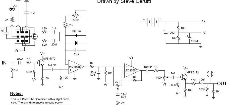
mod. The only difference is a round epoxy rectifier diode and 1N4148 instead of two 1N914 diodes in the feedback loop. Also the 560K resistors to Vr are 510K in the TS-9. The transistors are also different.
