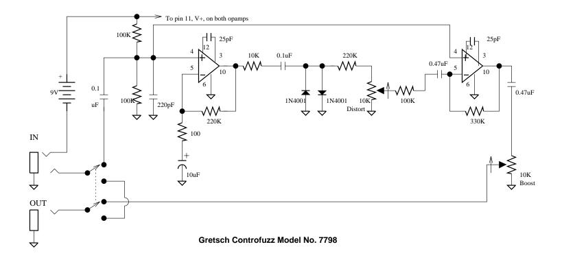
The Gretsch Controfuzz is a variant of the op-amp-driving-diode-clipper type of distorter. The only unusual features are that the distortion is run at high boost all the time in the first opamp, and then subtracted from the dry signal in the second opamp. The amount of distortion mixed in is determined by the "Distort" control, and the overall volume level when the distortion is switched in is set by the "Boost" control.
