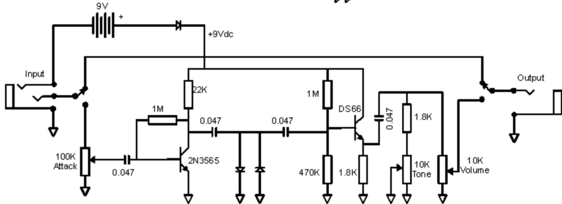
Diodes are unknown glass body diodes, probably silicon. DS66 is unknown type - but it's an emitter follower, so how hard can it be?
