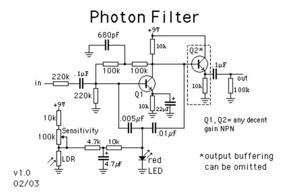
One implementation of the Idiot Wah, this version uses a LDR to control the wah. Makes a interesting pedal. Sensitivity pot allows useful control in dim or bright light. Variable resistance element is a LED to ground. The Q2 output buffer is nice to have, keeps the filter from getting loaded down at the output. But not absolutely necessary. The LDRs I have go down to about 1k in bright light, YMMV.
