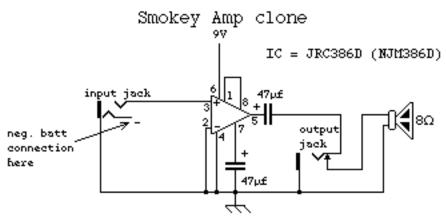
The JRC386D aka NJM386D (used in the Smokey) seems more stable and easier to tame than the National Semiconductor LM386. If yours is unstable, oscillates, or unusually yucky sounding, use the inverting input (pin 2) and ground the non-inverting input (pin 3). This may help. For less distortion, run at 12 Volts. for variable gain, put a switch between pins 1 and 8.
