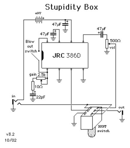
The Stupidity Box has evolved from a plain distortion box into a plain distortion/power amp. Works like a normal dist box, plug it into a speaker cab, crank the volume, and it's a high gain 1/2W power amp. The JRC386D (NJM386D) is a must in this circuit.
