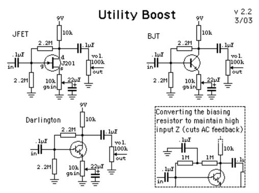
Simple booster/preamp for electric guitar or anything. J201 version is fairly clean even at max gain, high input Z, breaks up nicely. BJT version has lower input Z, more gain, breaks up more harshly (MPSA18, 2N3904, NTE103 tested). Darlington version is like BJT, high gain, breaks up harshly, but with higher input Z. Each circuit draws less than 500µA. Same circuit works with J201, MPSA18, 2N3904, NTE103, MPSA13, MPSA14.
