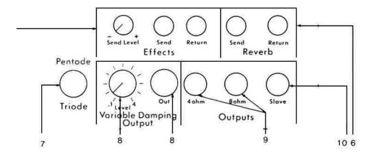
With the Standby switch in the up position, your amp will be on With the Standby switch in the down position, Standby will be in operation and no sound will come from the amp.
