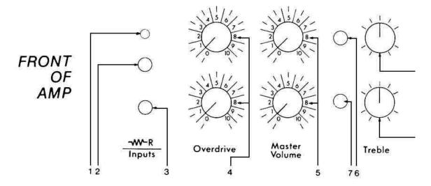
1) LOAD RESISTOR INPUT (Combo only) Guitar pickups have different output voltages. Using the load resistor plugs supplied with your combo amp, you can match your pickups to the amp's input.
