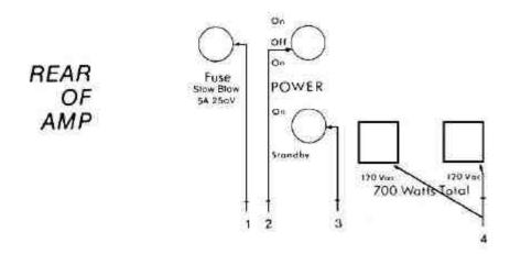
1) FUSE HOLDER: The fuse is located in the cap of the fuse holder. If the fuse fails, it must be replaced with one that provides proper current protection or you will void the warranty. The proper fuse rating for the 110-120 v.a.c. Convertible amp is 5A 250V slo blow.
